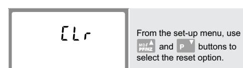
From the set-up menu, use **MDI/PPHZ** and **P** buttons to select the reset option.
